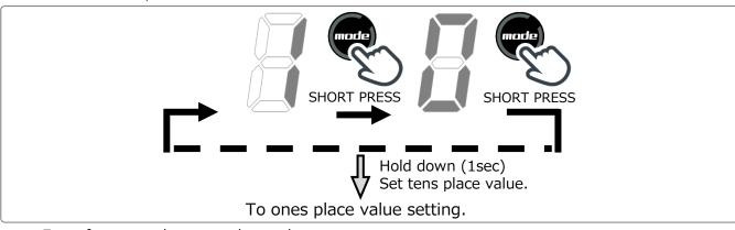
Enter front sprocket ones place value. In case of 14T, select 4. Hold down button to set.
