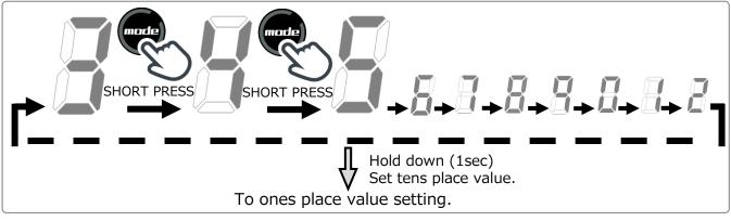
Enter rear sprocket ones place value. In case of 38T, select 8. Hold down button to set.
