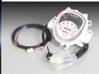
You can see what speed you are choosing by the meter for gear position indicator inside.
