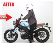
Protruding front fork as well as installing low down link plate is required.
