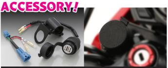
To prepare battery supply for mobile phone and etc. Just insert between couplers. No wiring mods required. Place it on accessory socket stay next to main key.
