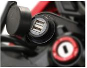
Uses accessory power (ACC+) The power and built-in LED (blue) is turned on when key is on.
