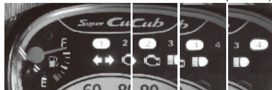
WINKER FI WARNING LAMP HIGH BEAM NEUTRAL
