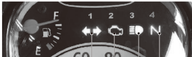
WINKER FI WARNING LAMP HIGH BEAM NEUTRAL
