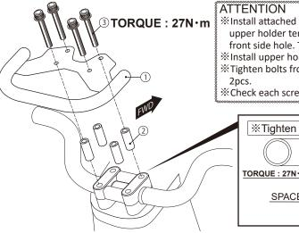
Install attached M8 bolt, aluminum collar and upper holder temporarily to multi purpose bar front side hole. Then install to vehicle.
