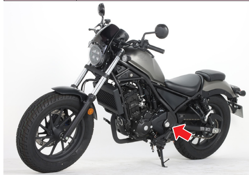
Just exchange with both side stock resin pivot bolts on frame!
