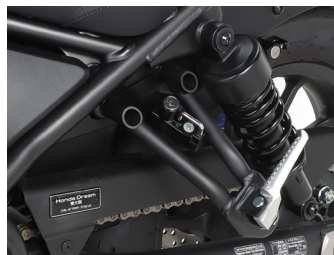
Helmet lock tightened with tandem step! Very convenient when touring / short time break.
